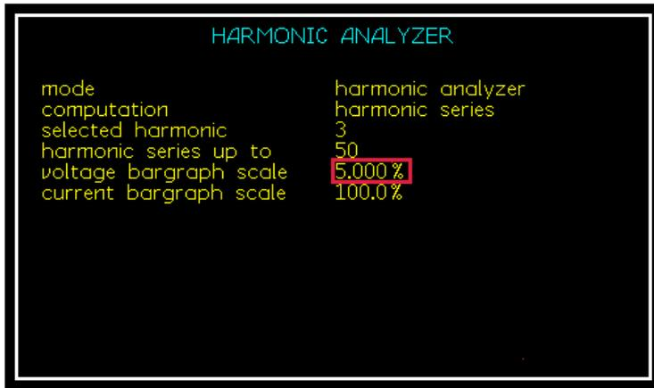
Press "GRAPH" to show the new bar graph results with the voltage results set to 5% of full voltage range as shown in Fig 10
