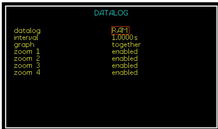
When the RAM option is selected: Use the ▼ key to step down to “interval” and enter the time between datalog measurements.
