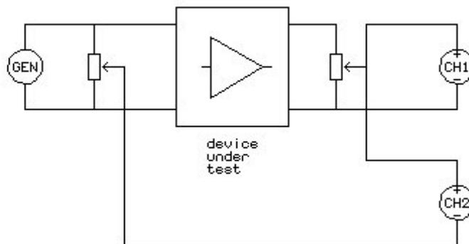
NB. only one attenuator is needed in any given test – use on the input if the forward gain of the DUT is 1 or lower, use on the out put if the gain is greater than 1. The attenuator should be of low impedance so that the capacitance of the leads and inputs does not filter the signal.
